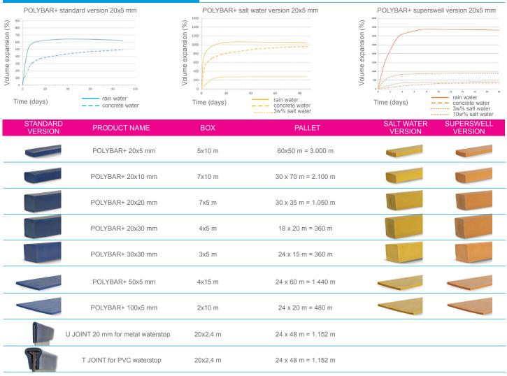
Polybar+ self-expanding sealing bars are based on a thermoplastic synthetic rubber and are available in :
